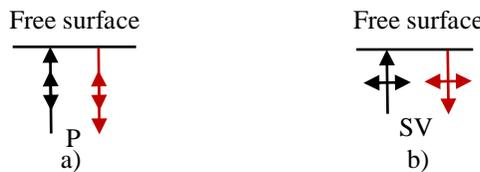
Figure 1. vertically incident waves a) P-wave b) SV-wave.
